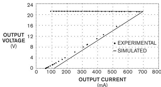
Figure 2 Simulated and measured foldback-current responses to a load resistance that varies from 200 to 0.01Ω show close agreement.
